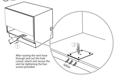
ALTERNATIVE METHOD (b) - SECURE BY DRAWER REMOVAL
